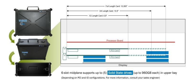
Note: Alternately, the upper storage area ("processor bay") can also be used for two additional quick-time removable drives.
