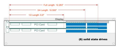
Note: Drives are stacked from the display side. So a full-length PCI card in slot 1 eliminates the ability to have any drives
