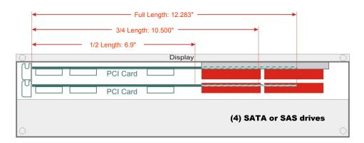
Note: Drives are stacked from the display side. So a full-length PCI card in slot 1 eliminates the ability to have any drives
