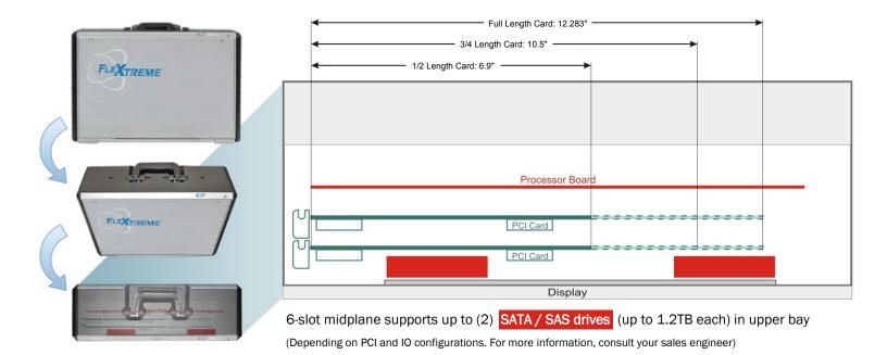
Note: Alternately, the upper storage area ("processor bay") can also be used for two additional quick-time removable drives.
